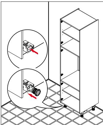
Prior to commencing kitchen installation work, check the delivered parts against the delivery note for completeness. Plug into leg receiver (s. illust.).
